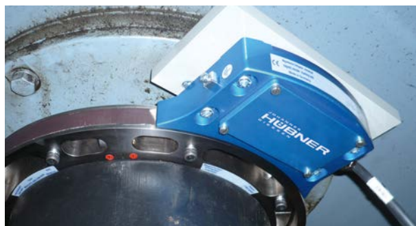
解体せずにスプリットパルスホイールで実現 Realization with split pulse wheel without dismantling of installation
